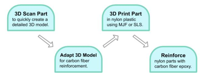
Carbon fiber-reinforced nylon replacement parts can be produced in a four-step process.
