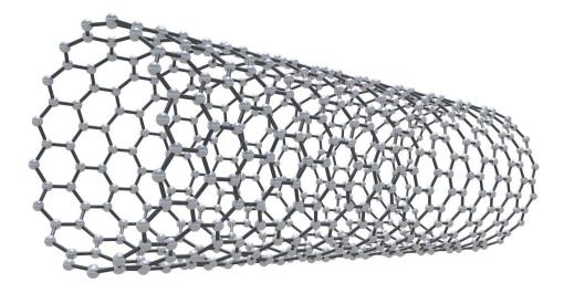
Carbon crystals create tubes that align in parallel strands to form carbon fibers.
